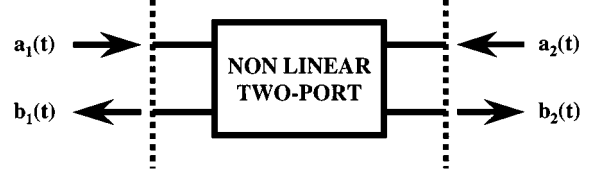
Fig. 4. Two-port nonlinear device described in the time domain.
